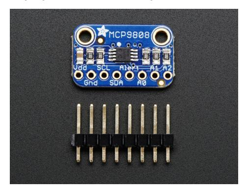
Unlike the DS18B20, this sensor does not come in through-hole package so we placed this small sensor on a breakout
