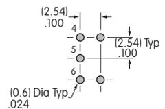
On single pole models positions 1 & 3 are support pins.
