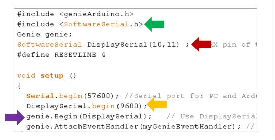
Refer to the product page of your Arduino board to know the pins that can be used for a software serial port. The section "**Connect the 4D Display Module to the Arduino Host**" towards the end of this application note shows how the TX and RX pins of the host are connected to those of the display. The following are the SoftwareSerial baud rates that were tested to work with 4D displays using the basic application that comes with this application note.
