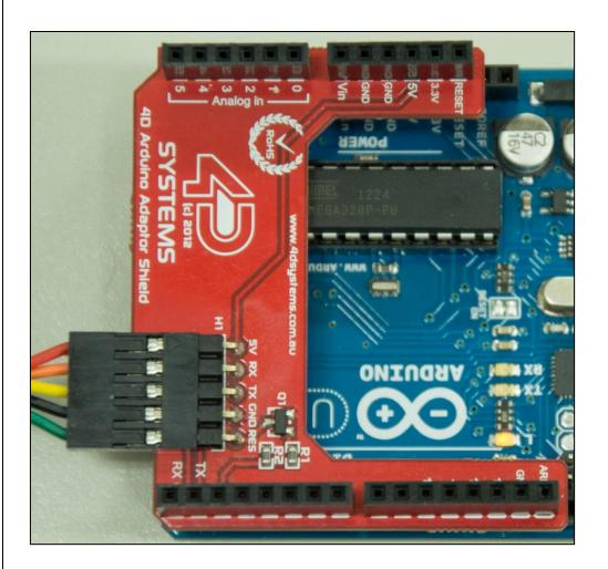
The old 4D Arduino Adaptor Shield (Rev1) uses digital pin **D2** for resetting the display. The reset routine of the Arduino sketch must be modified accordingly.
