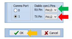
Compile and download the program to the display. All subsequent ViSi-Genie programs with a Diablo16 target display will now use COM1 with the specified TX and RX pins. Also, the TX and RX pins of the host shall now be connected to the specified RX and TX pins of COM1. If using a uLCD-35DT for example,
