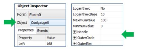
Feel free to experiment with the different properties. Take note of the maximum and minimum values. These determine the range of values that can be sent from the Arduino host to the cool gauge. To know more about gauges, refer to <u>ViSi-Genie Gauges</u>.
