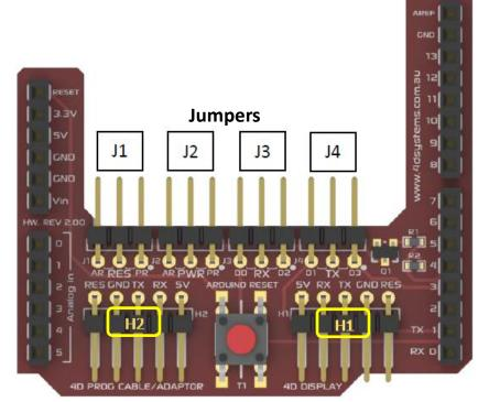
The 5-way cable coming from the display should be connected to **H1**. When the Arduino host cannot supply enough power to the display, the display can
