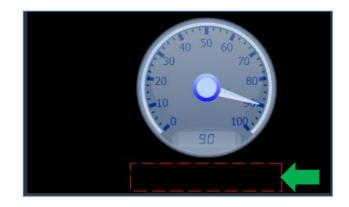
The space inside the red box will be the space occupied by the text string to be displayed. The object can be dragged to any desired location and resized to the desired dimensions. The **Object Inspector** on the right part of the screen displays all properties of the newly created strings object named **Strings0**.
