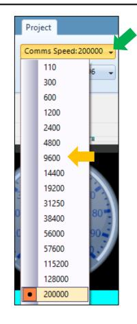
Choose the desired baud rate (9600 bps for instance) and download the program to the display module again. Now change the baud rate of the Arduino host as well.
