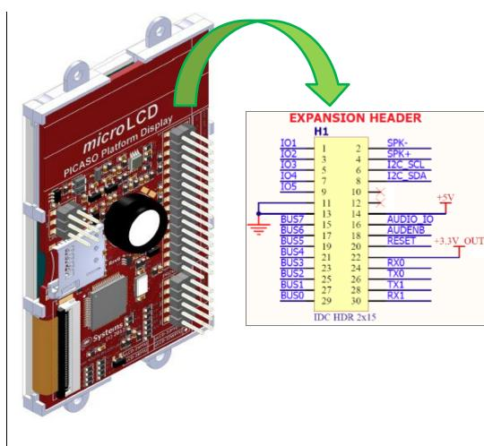
Note that the display here is powered off the **5V out** of the Arduino board. Pin **D4** of the host will also reset the display (logic of the reset routine must be inverted). Connect the **5V** and **GND** pins of the display to an external **5V** power supply source if a separate supply is needed. The reset pin, **RES**, of the display can also be connected to another GPIO pin of the Arduino host and the sketch can be modified accordingly.
