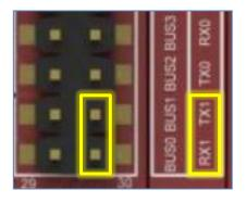
**The Diablo16 processor** has four serial ports – COM0, COM1, COM2, and COM3. The TX and RX pins of COM0 are fixed and are used for programming the processor. Again, COM0 is also the default serial port used by a ViSi-Genie program. The TX and RX pins for COM1, COM2, and COM3, on the other hand, are 'mappable' – that is, they can be configured to be 'mapped' out to any (but not all) of the GPIO pins. The table below shows the GPIO
