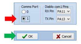
Compile and download the program to the display. All subsequent ViSi-Genie programs will now use COM1. Also, the TX and RX pins of the host shall now be connected to the RX and TX pins of COM1 instead of COM0.
