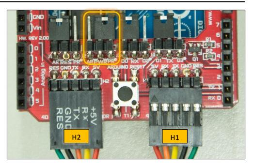
H2 is for the 4D USB Programming Cable or  $\mu$ USB-PA5 (power supply source), and H1 is for the display module. The following image shows how the Arduino host and the 4D display are connected when they are powered separately.
