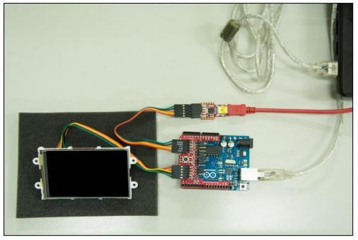
Note that the display module cannot be programmed thru the  $\mu$ USB-PA5 in this setup since H2 transfers power only. Before programming the display module, disconnect it first from the Arduino Adaptor Shield. Likewise, before programming the Arduino host, make sure that it is not connected to the display module. Do this when the communication is thru **Serial0** (Arduino host) and **COM0** (4D display). Always double check the orientation of the connections.
