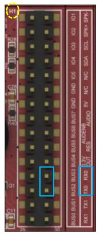
As the reader may have already perceived, the TX and RX pins on the programming header are the same pins as TXO and RXO on the H1 I/O expansion header. In Workshop it is possible to change the serial port being used by a ViSi-Genie program. Instructions for doing this are as follows.
