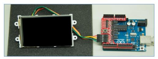
Using the jack(the Arduino host powers the display):
